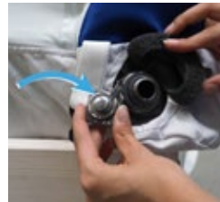
Photo 15: Open front cap of valve.
